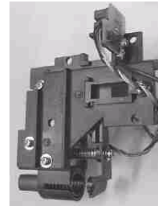
Figure 4-45. Cutter Housing Removal 2/2
