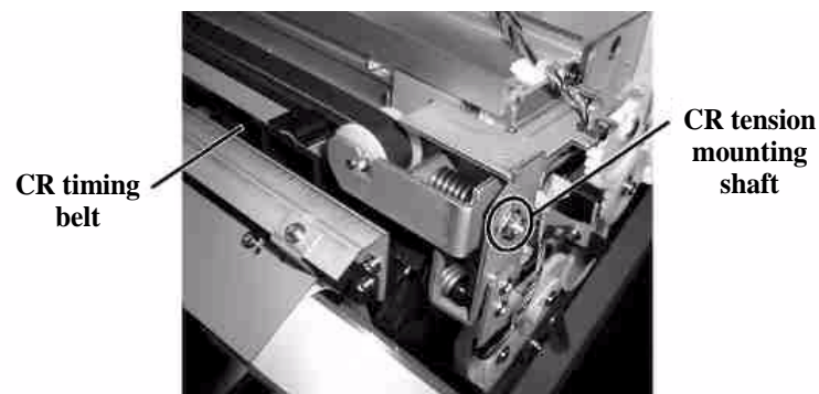
Figure 4-61. Loosening the CR Tension Belt
