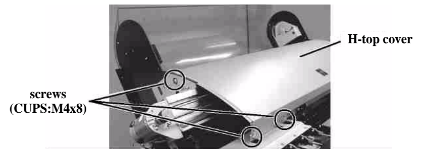
Figure 4-14. H Top Cover Removal on left side
