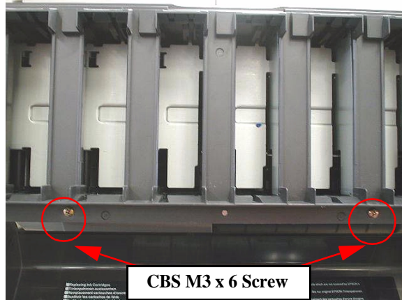
Figure 4-126. Removing the I/H Cover
