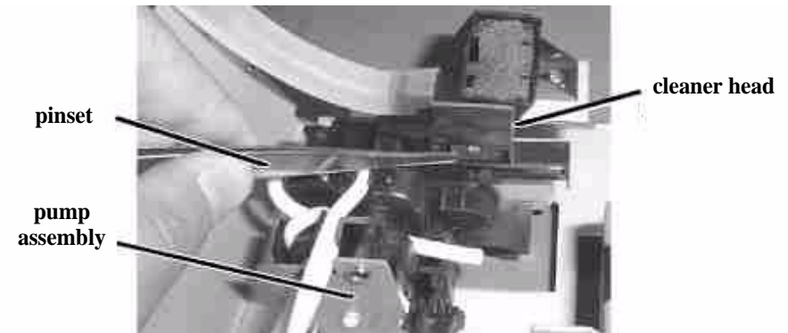
Figure 4-82. Removing the Cleaner Head
