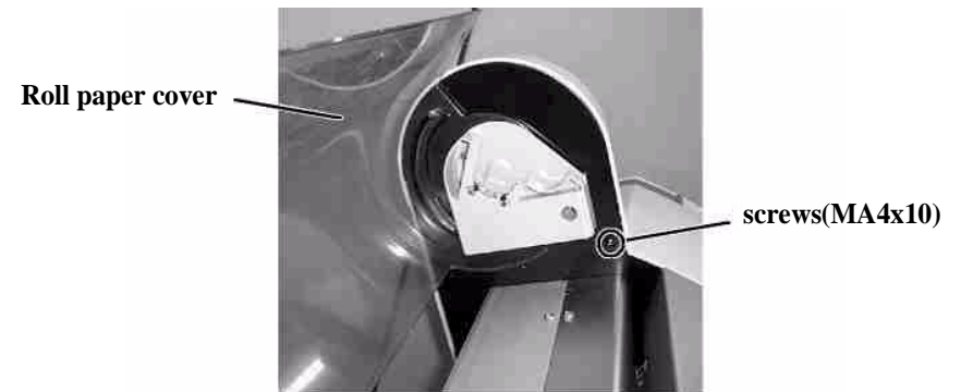
Figure 4-7. R Side Cover Removal 2/4
